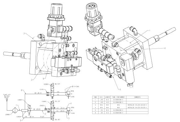
Figure 42: PR70 Air Cylinder System and Schematic
